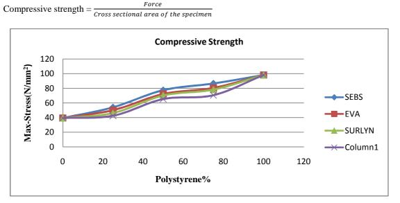
**Figure 3: Compressive Strength at Different Compatibilizers** (5% w/w) and Different PS/PP Compositions
