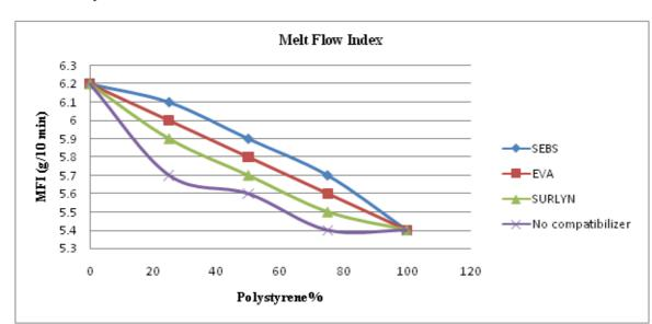
Melt Flow Index =  $\frac{600 \cdot M}{t}$ , (gm/10min) Where, M = avg. mass, gm t = cut- off time, min
