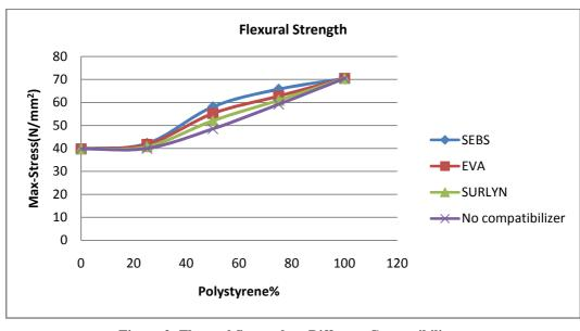
**Figure 2: Flexural Strength at Different Compatibilizers** (5% w/w) and Different PS/PP Compositions
