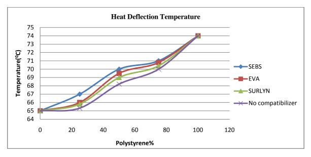
Figure 5: HDT at Different Compatibilizers (5% w/w) and Different PS/PP Compositions
